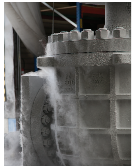
In-house full range cryogenic testing
